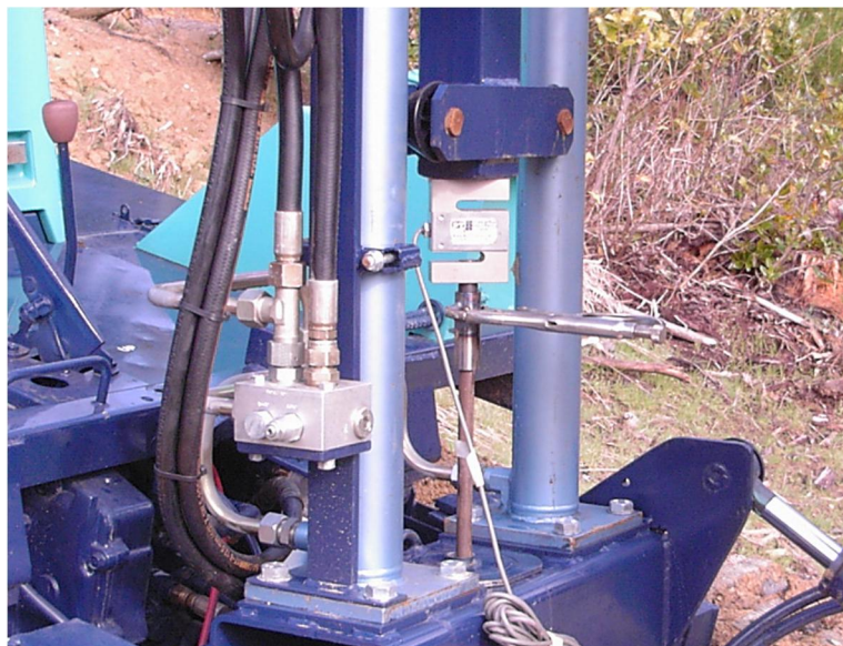
Figure 2. View of electric load cell at top of push rods.
